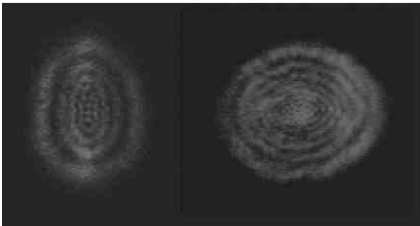
The left side of the image shows the defocused disk of a star with a focussers position shifted inside (infocal) with respect to the sharp image (focal) and the right image shows this defocused disk for an focussers position outside of focus (extrafocal). The images might also be reversed, with the left image corresponding to the extrafocal position and the right image to the infocal position.
