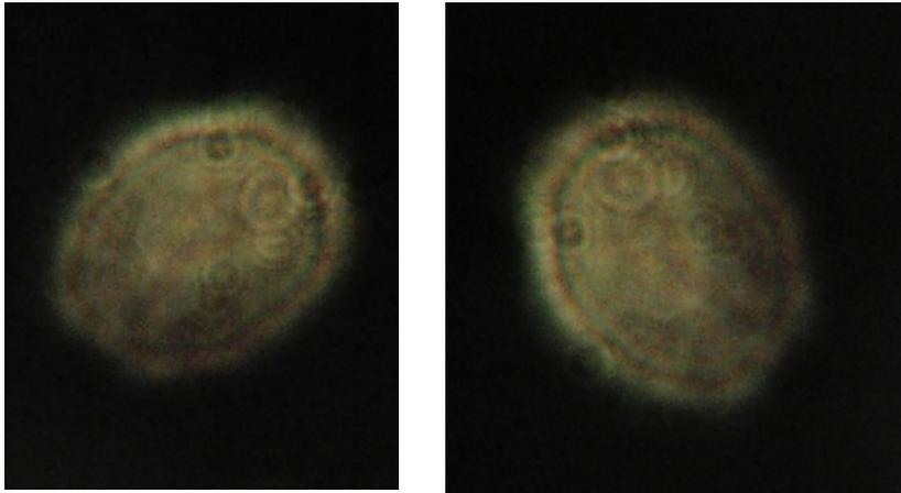
The left side of the image shows the defocused disk of a star with a focussers position shifted inside (infocal) with respect to the sharp image (focal) and the right image shows this defocused disk for an focussers position outside of focus (extrafocal). The images can also be reversed - with the left image corresponding to the extrafocal position and the right image to the infocal position of the focusser.
