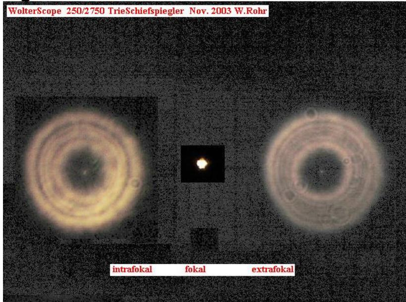
The left and right side of the image show the defocused disk of a star with a focussers position shifted inside with respect to the sharp image (focal) and outside of focus. In the center of Fig. 3 you see the Airy disk of the focused star. The corresponding diffraction rings are not resolved in this image.
